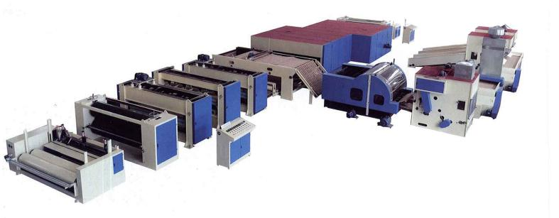
The production line is a combination for making glue free wadding and needle punching felt.
